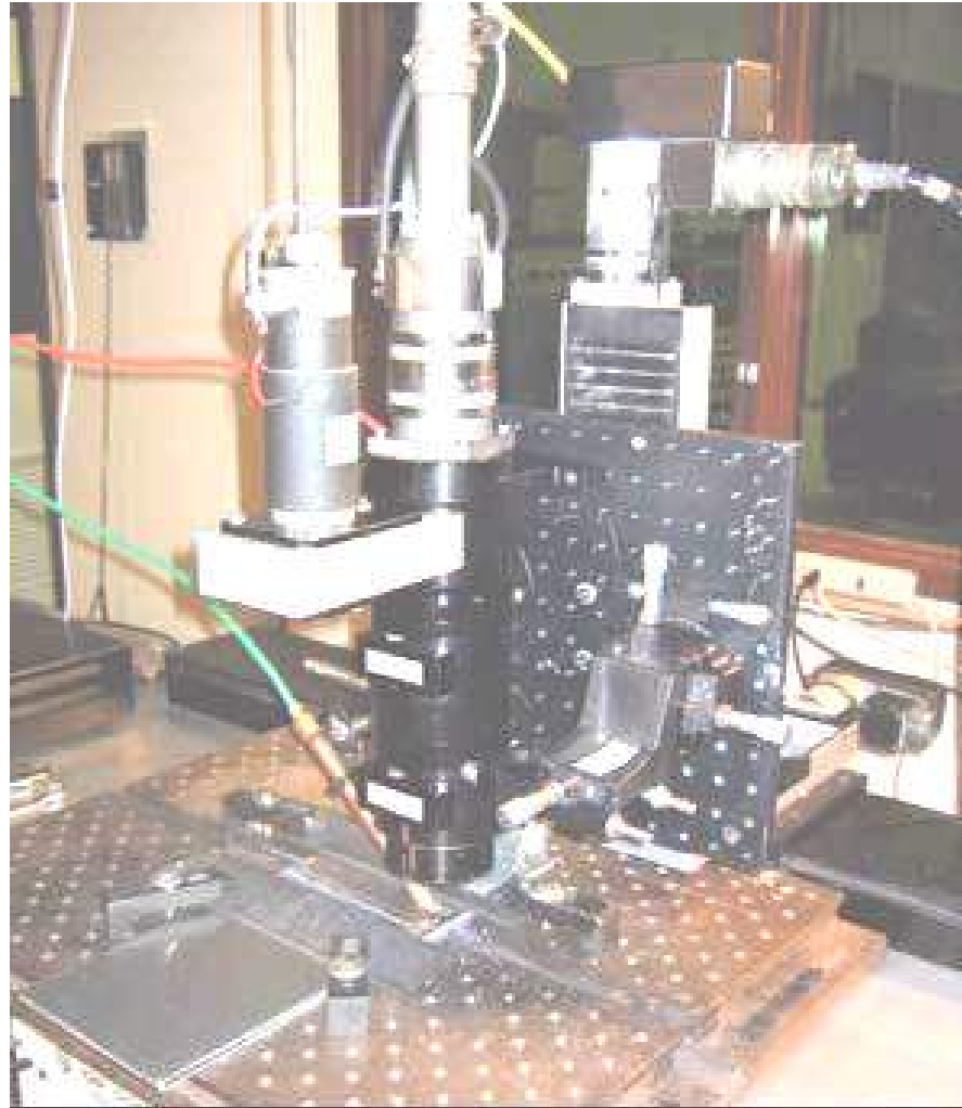
Experimental apparatus for laser stir welding (Martukanitz and Tressler, 2006).
