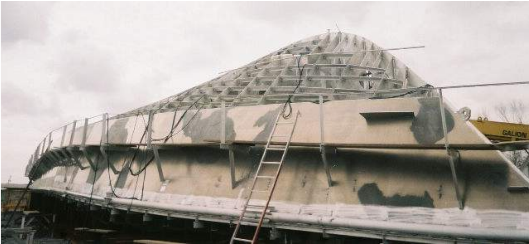
Hull with stick construction of framing (Courtesy of Gulf Craft)
