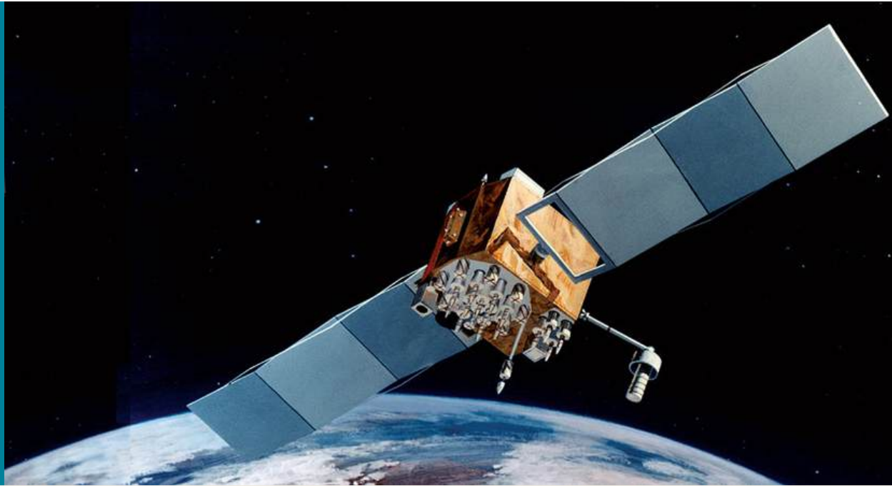
Figure 5.1 Special relativity explains how time passes slightly differently on Earth and within the rapidly moving global positioning satellite (GPS). GPS units in vehicles could not find their correct location on Earth without taking this correction into account. (credit: modification of work by U.S. Air Force)
