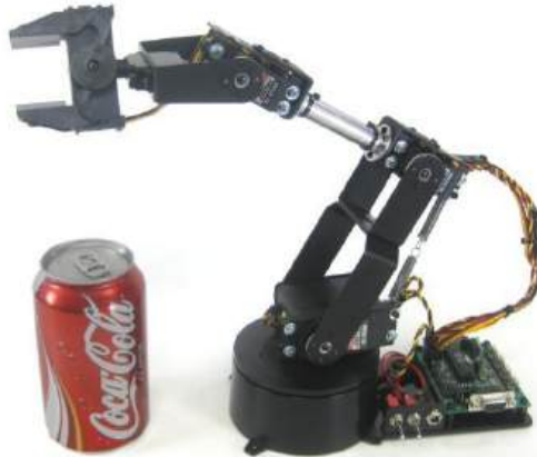
Figure 12.3 4 DOF arm robot using stereo vision used in the experiment.
