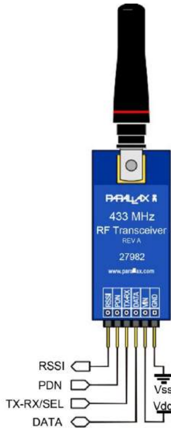
Figure 4.4 Wireless communication using 433 MHz Transceiver.
