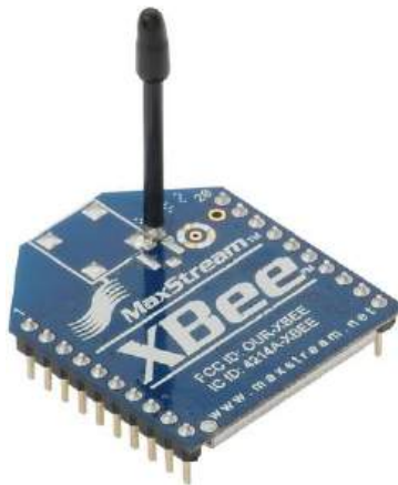
Figure 4.5 Wireless communication using XBee.
