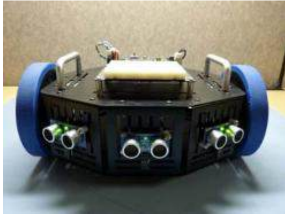
Figure 3.9 Avoider robot using 3 PING))) on the body.
