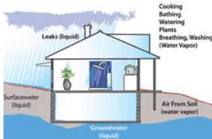
Fig. 73 Demonstration how humidity formed in building
