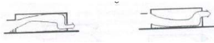
Fig.110 How canopies effect ventilations
