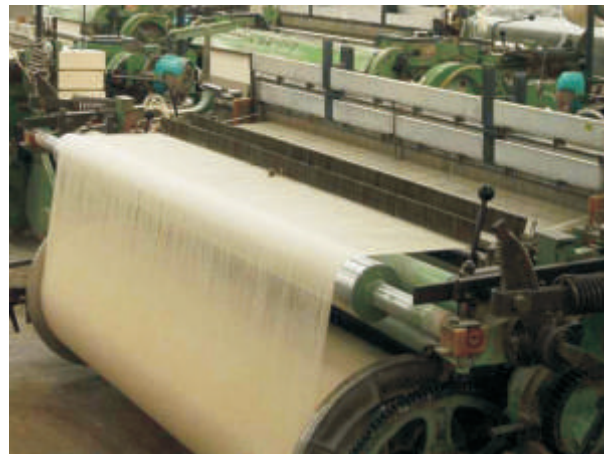
Fig 30: Fabric being woven on a powerloom
