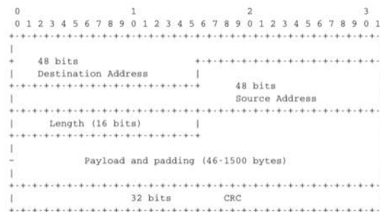
Figure 6.21: Ethernet 802.3 frame format
