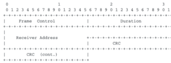
Figure 6.35: IEEE 802.11 ACK and CTS frames
