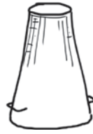
cone for slump test
