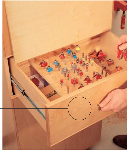
Drill the \frac{1}{2} " and \frac{1}{4} " holes. Nail in a couple of rails on the inside of the drawer and simply drop the panels in place. The panel for \frac{1}{2} "-shank bits is drilled all the way through and the panel for \frac{1}{4} "-shank bits is drilled down \frac{5}{8} ".
