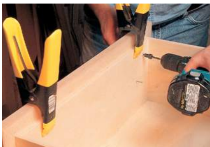
After attaching the slide to the drawer, mark the location of the cabinet part of the slide on the cabinet side. Use a framing square to run a line back from this mark and mount the slide \frac{1}{16} " back from the front of the cabinet.
