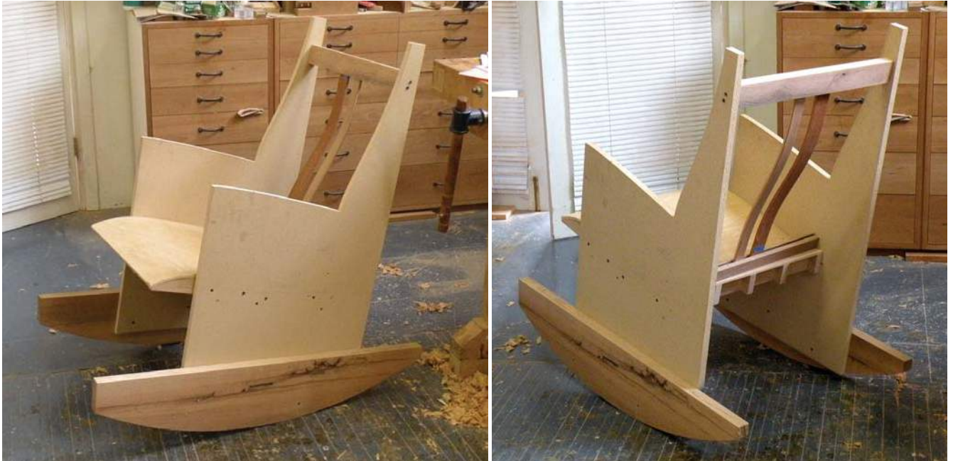
Mock you to sleep. This mock-up of my rocker design allowed me to quickly change variables and immediately feel the outcome.
