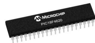
Figure 3.1.7: A PIC microcontroller. (Source: Microchip )
