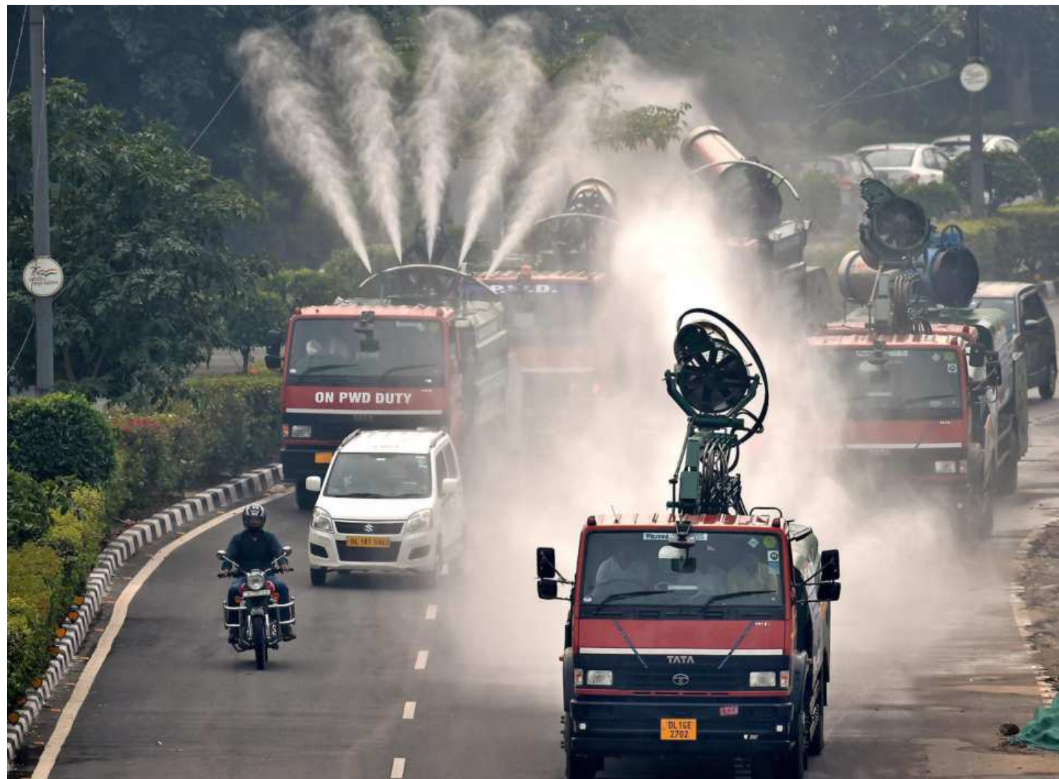
The Delhi government launched 50 mobile 'anti-smog guns' in response to the national capital's dreadful air quality, on Tuesday. The guns spray nebulised water to absorb dust and contaminants from the air, but their efficacy is unproven. SHASHI SHEKHAR KASHYAP
