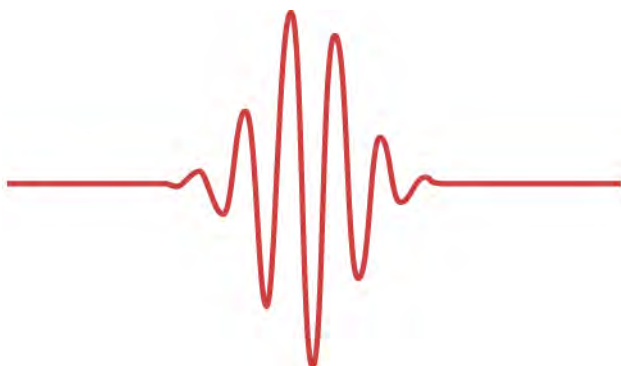
Figure 6.25 In this graphic, a particle is shown as a wave packet and its position does not have an exact value.
