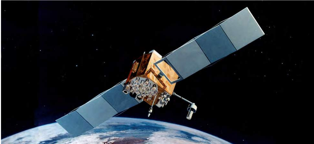
Figure 5.1 Special relativity explains how time passes slightly differently on Earth and within the rapidly moving global positioning satellite (GPS). GPS units in vehicles could not find their correct location on Earth without taking this correction into account. (credit: modification of work by U.S. Air Force)
