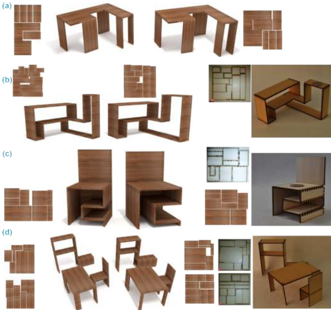
Fig. 11. Various material-driven design and fabrication examples. In each row, we show initial design (with material space layout inset), optimized design result (with material space layout inset), along with final cutout assembled model. Note that the design changes are often subtle, but still leads to significant improvement in material usage.
