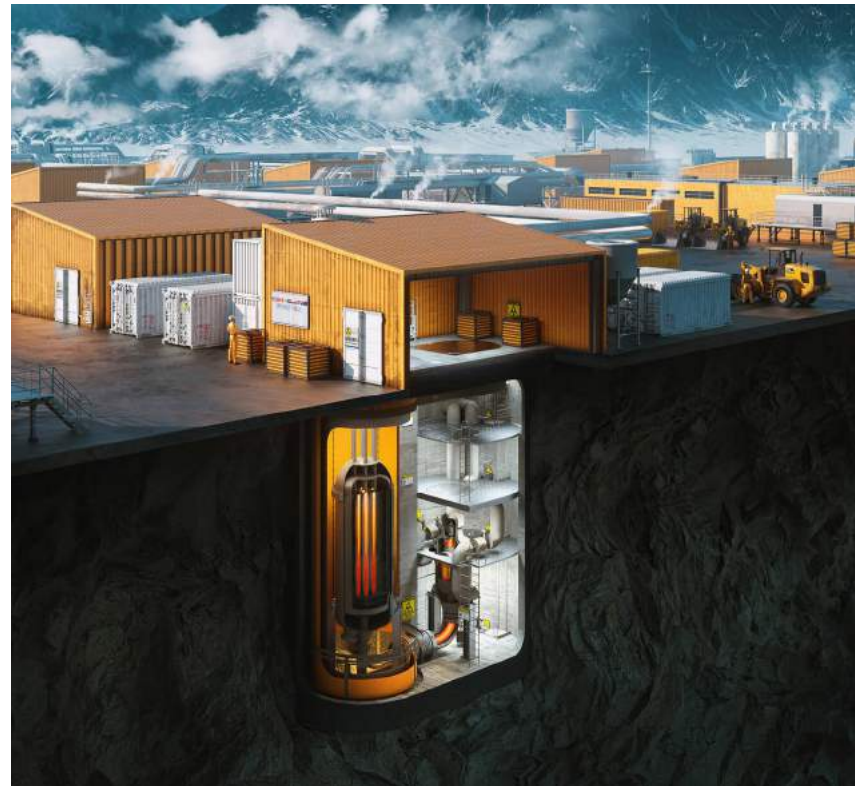
Figure 8 Example of a microreactor: schematic of Ultra Safe Nuclear Corporation's micro modular reactor
