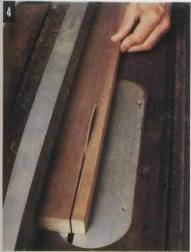
4 Rip the walnut into 1¾" strips and cut them into four 18" lengths.
