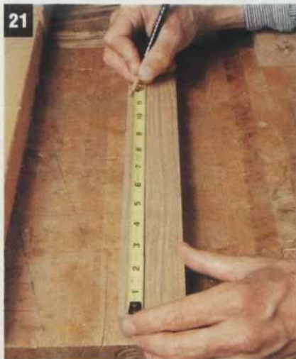
Measure an 11½" length on the 1" x 2" x 48" skirt piece. Square the mark and cut. Repeat for the remaining three skirt pieces. Now's the time to check the skirts and legs for blade burn, and sand the faces if needed.
