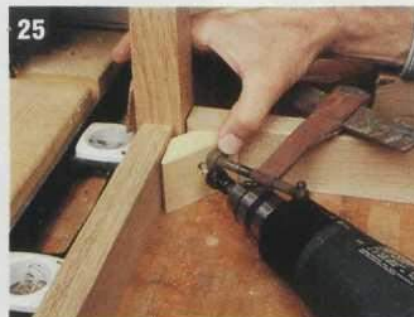
Set up the table frame on a flat work surface with a band clamp placed snugly around the frame's circumference. Use a #6 screw bit with the stop collar set at 1¾" to pre-drill a hole through each brace and then into the leg behind it. Center the hole ¾" from the exposed edge, and set the braces flush against the work table.
