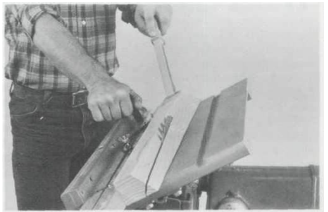
Triangle formed by saw kerf and blade should be 3/4" on each side. (Saw guard removed for clarity only.)
