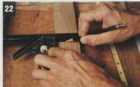
Measure an 11½" length on the 1" x 2" x 48" skirt piece. Square the mark and cut. Repeat for the remaining three skirt pieces. Now's the time to check the skirts and legs for blade burn, and sand the faces if needed.
