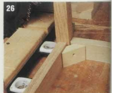
Glue the skirts to the legs, and the braces to the skirts. If the corner braces don't set squarely against the skirts, place and draw up the cabinet screws lightly to hold the braces in place. Tighten the band clamp.
