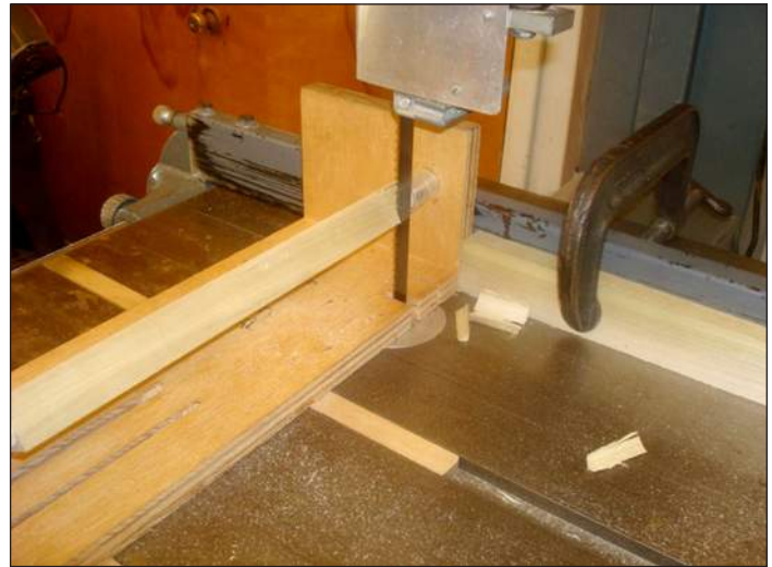
Trimming the tenons on a band saw with a jig
