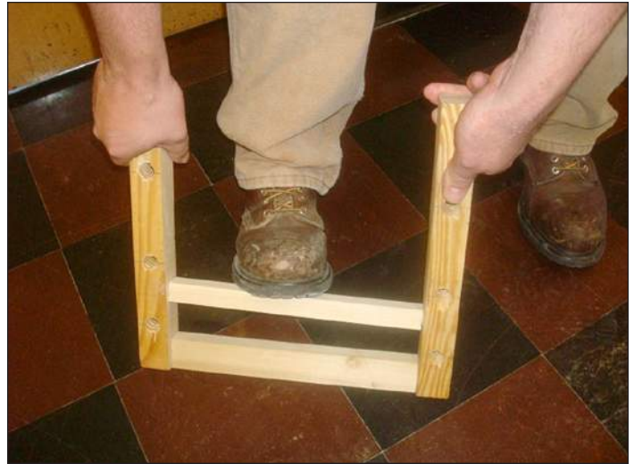
Method for twisting front legs so they lay flat
