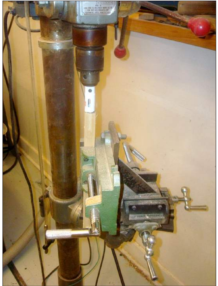
Drill press setup with cross-slide vise, angle plate, and vertical vise
