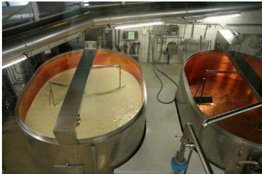
Figure 16.3.2 Industrial cheese production. 10,000 l milk in the left tank, the milk was mixed with rennet and is now broken for the production of Emmentaler.. (CC BY-SA 3.0; MatthiasKabel ).
