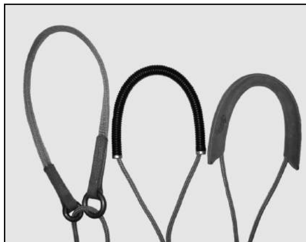
Figure 5c: (left to right) Ring and ring, conduit sleeve, leather sleeve friction savers.
