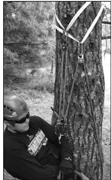
Figure 8c: Z-rig pulley system
