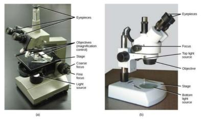
**Figure 3.2** (a) Most light microscopes used in a college biology lab can magnify cells up to approximately 400 times. (b) Dissecting microscopes have a lower magnification than light microscopes and are used to examine larger objects, such as tissues.
