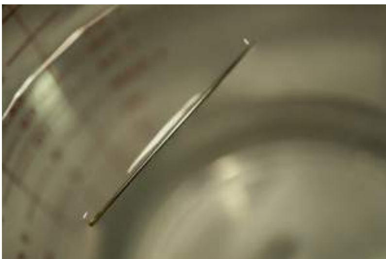
Figure 2.10 The weight of a needle on top of water pulls the surface tension downward; at the same time, the surface tension of the water is pulling it up, suspending the needle on the surface of the water and keeping it from sinking. Notice the indentation in the water around the needle.
