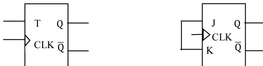
Figure: 3. 6a) Block Diagram of T flip-flop b) T flip-flop using a J-K flip-flop
