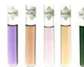
Figure 21.2.3 Compounds of Manganese in Oxidation States +2 to +7 Like vanadium, compounds of manganese in different oxidation states have different numbers of d electrons, which leads to compounds with different colors: the \text{Mn}^{2+}(\text{aq}) ion is pale pink; \text{Mn}(\text{OH})_3 , which contains Mn(III), is a dark brown solid; \text{MnO}_2 , which contains Mn(IV), is a black solid; and aqueous solutions of Mn(VI) and Mn(VII) contain the green manganate ion [\text{MnO}_4]^{2-} and the purple permanganate ion [\text{MnO}_4]^- , respectively.
