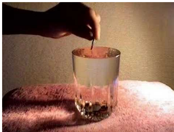
Figure 11.3.2 The Effects of the High Surface Tension of Liquid Water (a) A paper clip can “float” on water because of surface tension (from Christopher Rozitis ).
