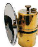
19th-century miner's lamp. The lamp uses burning acetylene, produced by the slow reaction of calcium carbide with water, to provide light.
