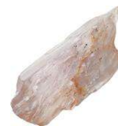
A crystal of spodumene ( LiAlSi_2O_6 ). This mineral is one of the most important lithium ores.
