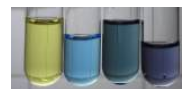
Figure 21.2.2 Aqueous Solutions of Vanadium Ions in Oxidation States of +2 to +5 Because vanadium ions with different oxidation states have different numbers of d electrons, aqueous solutions of the ions have different colors: in acid V(V) forms the pale yellow [VO_2]^+ ion; V(IV) is the blue vanadyl ion [VO]^{2+} ; and V(III) and V(II) exist as the hydrated V^{3+} (blue-green) and V^{2+} (violet) ions, respectively.
