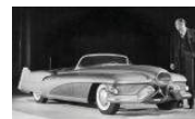
Figure 20.4.1 Magnesium Alloys Are Lightweight and Corrosion Resistant Because magnesium is about five times lighter than steel and 50% lighter than aluminum, it was long considered the “material of the future,” as shown in this 1950 concept Buick LeSabre sports car made almost entirely of magnesium and aluminum alloys. Modern aluminum alloys usually contain about 5% magnesium to improve their corrosion resistance and mechanical properties.
