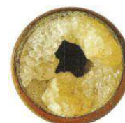
Figure 13.4.3 Boiler Scale in a Water Pipe Calcium carbonate ( \text{CaCO}_3 ) deposits in hot water pipes can significantly reduce pipe
