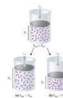
Figure 18.1.3 PV Work Using a frictionless piston, if the external pressure is less than P_{\text{int}} (a), the ideal gas inside the piston will expand, forcing the piston to perform work on its surroundings. The final volume ( V_f ) will be greater than V_i . Alternatively, if the external pressure is greater than P_{\text{int}} (b), the gas will be compressed, and the surroundings will perform work on the system.
