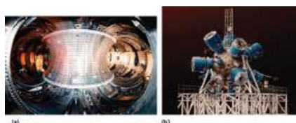
Figure 24.5.4 Two Possible Designs for a Nuclear Fusion Reactor The extraordinarily high temperatures needed to initiate a nuclear fusion reaction would immediately destroy a container made of any known material. (a) One way to avoid contact with the container walls is to use a high-energy plasma as the fuel. Because plasma is essentially a gas composed of ionized particles, it can be confined using a strong magnetic field shaped like a torus (a hollow donut). (b) Another approach to nuclear fusion is inertial confinement, which uses an icosahedral array of powerful lasers to heat and compress a tiny fuel pellet (a mixture of solid LiD and LiT) to induce fusion.
