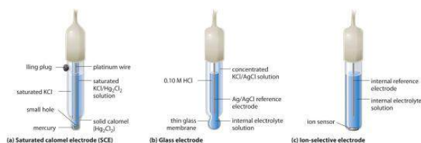
Figure 19.2.5 Three Common Types of Electrodes: (a) The SCE is a reference electrode that consists of a platinum wire inserted into a moist paste of liquid mercury (calomel; Hg_2Cl_2 ) and KCl. The interior cell is surrounded by an aqueous KCl solution, which acts as a salt bridge between the interior cell and the exterior solution. (b) In a glass electrode, an internal Ag/AgCl electrode is immersed in a 1 M HCl solution that is separated from the sample solution by a very thin glass membrane. The potential of the electrode depends on the H^+ ion concentration of the sample. (c) The potential of an ion-selective electrode depends on the concentration of only a single ionic species in solution.
