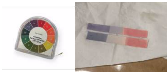
Figure 16.5.9 pH Paper pH paper contains a set of indicators that change color at different pH values. The approximate pH of a solution can be determined by simply dipping a paper strip into the solution and comparing the color to the standards provided.
