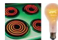
Figure 2.2.1 Blackbody Radiation When heated, all objects emit electromagnetic radiation whose wavelength (and color) depends on the temperature of the object. A relatively low-temperature object, such as an electric stove element, on a low setting appears red, whereas a higher-temperature object, such as the filament of an incandescent light bulb, appears yellow or white.
