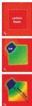
Figure 18.3.5 Thermograms Showing That Heat Is Absorbed from the Surroundings When Ice Melts at 0°C By convention, a thermogram shows cold regions in blue, warm regions in red, and thermally intermediate regions in green. When an ice cube (the system, dark blue) is placed on the corner of a square sample of low-density carbon foam with very high thermal conductivity, the temperature of the foam is lowered (going from red to green). As the ice melts, a temperature gradient appears, ranging from warm to very cold. An arrow indicates the direction of heat flow from the surroundings (red and green) to the ice cube. The amount of heat lost by the surroundings is the same as the amount gained by the ice, so the entropy of the universe does not change.
