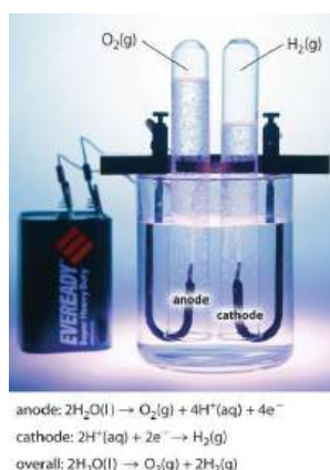
Figure 19.7.3 The Electrolysis of Water Applying an external potential of about 1.7–1.9 V to two inert electrodes immersed in an aqueous solution of an electrolyte such as H 2 SO 4 or Na 2 SO 4 drives the thermodynamically nonspontaneous decomposition of water into H 2 at the cathode and O 2 at the anode.
