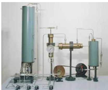
The original laboratory apparatus designed by Fritz Haber and Robert Le Rossignol in 1908 for synthesizing ammonia from its elements. A metal catalyst bed, where ammonia was produced, is in the large cylinder at the left. The Haber-Bosch process used
