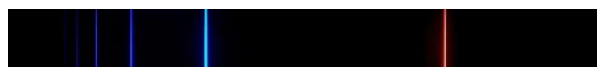
Figure 2.3.1 The Emission of Light by Hydrogen Atoms (a) A sample of excited hydrogen atoms emits a characteristic red light. (b) When the light emitted by a sample of excited hydrogen atoms is split into its component wavelengths by a prism, four characteristic violet, blue, green, and red emission lines can be observed, the most intense of which is at 656 nm.
