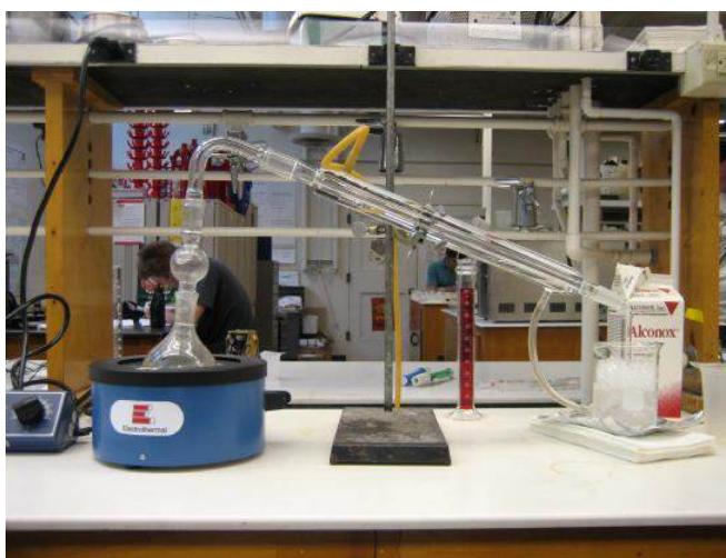
Figure 1.3.3 The Distillation of a Solution The solution of salt in water is heated in the distilling flask until it boils. The resulting vapor is enriched in the volatile component (water), which condenses to a liquid in the cold condenser and is then collected in the receiving flask.
