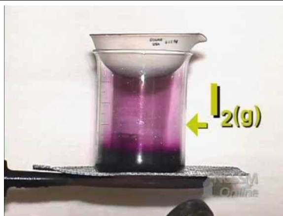
Figure 11.5.2 The Sublimation of Solid Iodine When solid iodine is heated at ordinary atmospheric pressure, it sublimates. When the I_2 vapor comes in contact with a cold surface, it deposits I_2 crystals.
