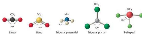
Figure 6.3.1 Common Structures for Molecules and Polyatomic Ions That Consist of a Central Atom Bonded to Two or Three Other Atoms
