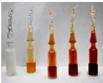
Figure 15.5.4 The Effect of Temperature on the Equilibrium between Gaseous \text{N}_2\text{O}_4 and \text{NO}_2 The value of K changes with temperature of the same 99.9% pure \text{NO}_2/\text{N}_2\text{O}_4 sealed in an ampoule. From left to right -196^\circ \text{C} , 0^\circ \text{C} , 23^\circ \text{C} , 35^\circ \text{C} , 50^\circ \text{C} . In the endothermic reaction, the equilibrium position can be shifted by changing the temperature. When heat is added and the temperature increases, the reaction shifts to the right and the flask turns reddish brown due to an increase in \text{NO}_2 . When heat is removed and the temperature decreases, the reaction shifts to the left and flask turns colorless due to an increase in \text{N}_2\text{O}_4 . This demonstrates Le Chatelier's Principle because the equilibrium shifts in the direction that consumes energy. Figure used with permission from Wikipedia.
