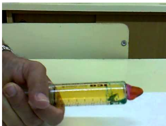
Figure 15.5.3 The Effect of Changing the Volume (and Thus the Pressure) of an Equilibrium Mixture of N_2O_4 and NO_2 at Constant Temperature (a) The syringe with a total volume of 15 mL contains an equilibrium mixture of N_2O_4 and NO_2 ; the red-brown color is proportional to the NO_2 concentration. (b) If the volume is rapidly decreased by a factor of 2 to 7.5 mL, the initial effect is to double the concentrations of all species present, including NO_2 . Hence the color becomes more intense. (c) With time, the system adjusts its composition in response to the stress as predicted by Le Châtelier's principle, forming colorless N_2O_4 at the expense of red-brown NO_2 , which decreases the intensity of the color of the mixture.
