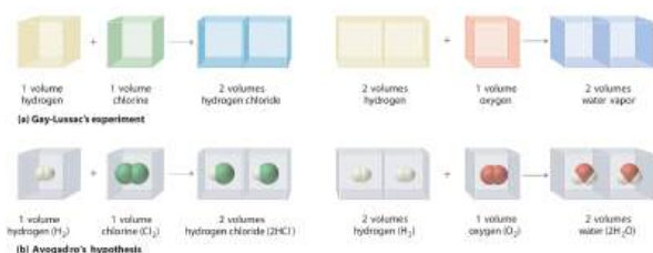
Figure 1.4.2 Gay-Lussac's Experiments with Chlorine Gas and Hydrogen Gas (a) One volume of chlorine gas reacted with one volume of hydrogen gas to produce two volumes of hydrogen chloride gas, and one volume of oxygen gas reacted with two volumes of hydrogen gas to produce two volumes of water vapor. (b) A summary of Avogadro's hypothesis, which interpreted Gay-Lussac's results in terms of atoms. Note that the simplest way for two molecules of hydrogen chloride to be produced is if hydrogen and chlorine each consist of molecules that contain two atoms of the element.
