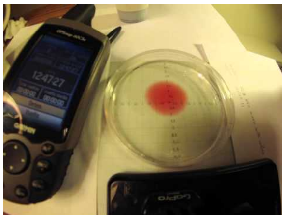
Figure 11.0.1 Molecular Diffusion in a Liquid A drop of an aqueous solution containing a marker dye is added to a larger volume of water. As it diffuses, the color of the dye becomes fainter at the edges.
