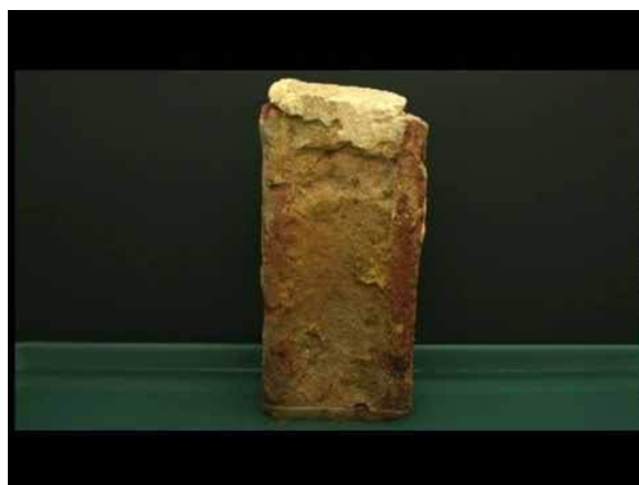
Figure 11.3.4 The Phenomenon of Capillary Action: Water rises through a brick in a time lapse video
