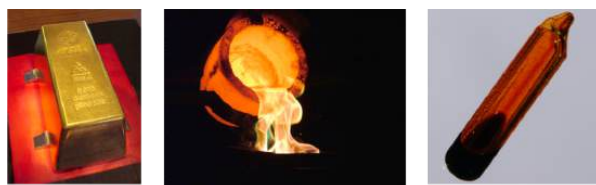
Figure 1.3.1 The Three States of Matter Solids have a defined shape and volume. Liquids have a fixed volume but flow to assume the shape of their containers. Gases completely fill their containers, regardless of volume. A bar of gold is shown to the left, liquid gold being poured in the center, and an ampule of liquid bromine with gaseous bromine at the right
