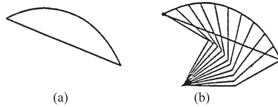
Figure 3.3.2: Comparison of trajectory linear interpolations in joint space and in cartesian space
