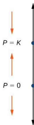
Figure 6.4.2: A phase line for the differential equation \frac{dP}{dt} = rP \left( 1 - \frac{P}{K} \right) .
