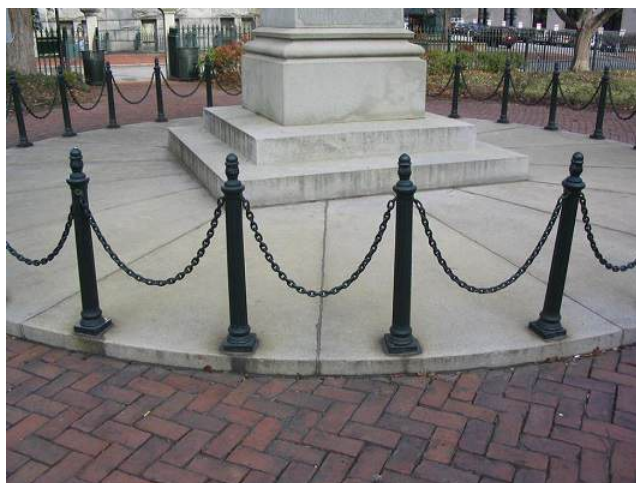
Figure 5.8.3: Chains between these posts take the shape of a catenary. (credit: modification of work by OKFoundryCompany, Flickr)
