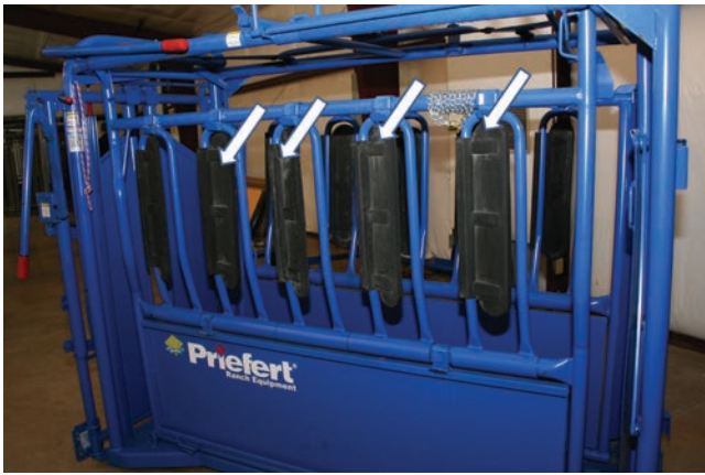
FIGURE 11-4. Flexible poly blinders to help funnel cattle into the headgate by reducing visual distractions from outside the chute.
