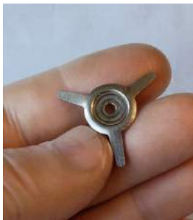
Figure 91 – three-legged friction spring
