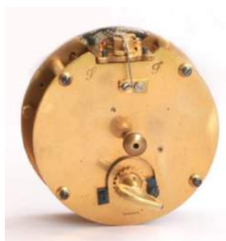
Figure 20 – drum movement showing platform escapement
