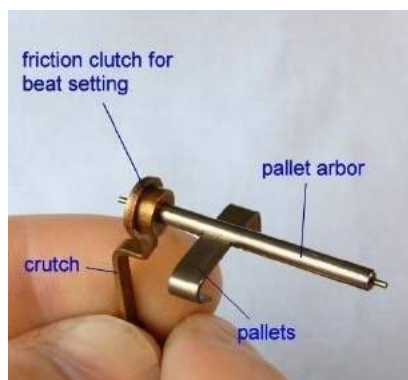
Figure 69 – pallet assembly
