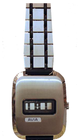
Figure 50 – very early LCD watch with "random dispersal" display
