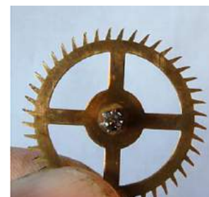
Figure 88 – tooth form of escape wheel
