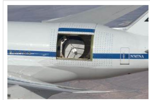
SOFIA is an infrared telescope in an aircraft, shown here in a 2009 test
