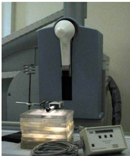
FIG. 22.5. Measurement of entrance surface air kerma using a PMMA slab. Note that the dosimeter and control unit are both shown in the photograph for demonstration purposes. In an actual situation, they would be further apart and the cable would not be coiled.
