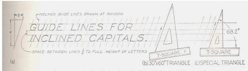
Figure 3.4 Guide lines for inclined capital letters
