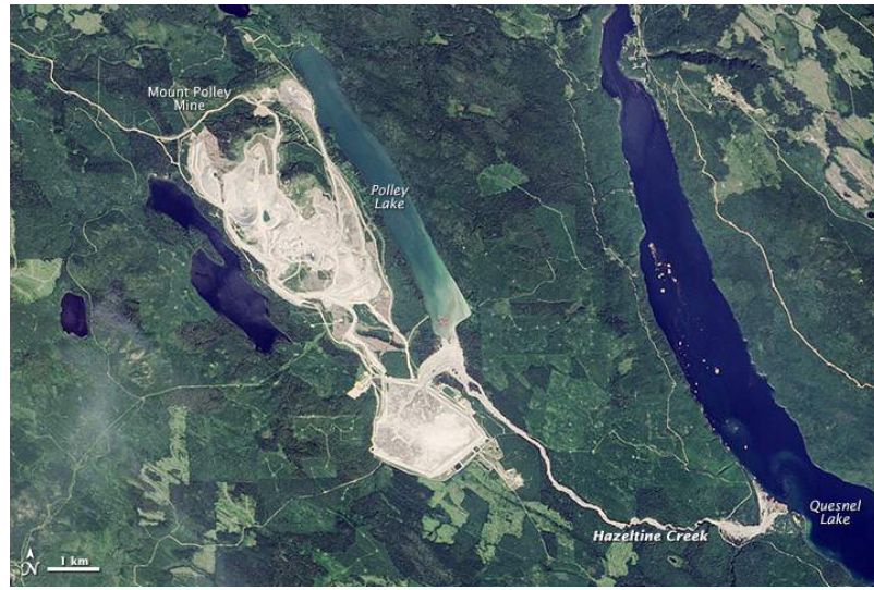
Figure 20.14b The Mt. Polley Mine area after the tailings dam breach of August 2014. The water and tailings released flowed into Hazeltine Creek, and Polley and Quesnel Lakes. [ https://en.wikipedia.org/wiki/Mount_Polley_mine_disaster ]
