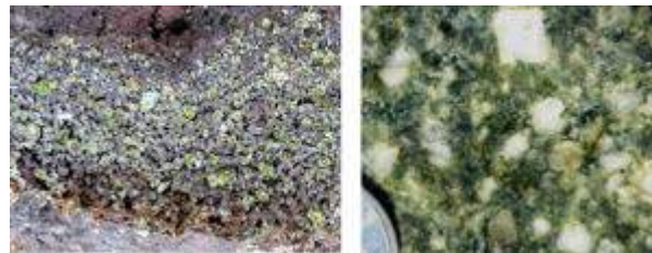
Figure 3.15 Porphyritic textures: volcanic porphyry (left – olivine crystals in Hawaiian basalt) and intrusive porphyry (right) [SE]
