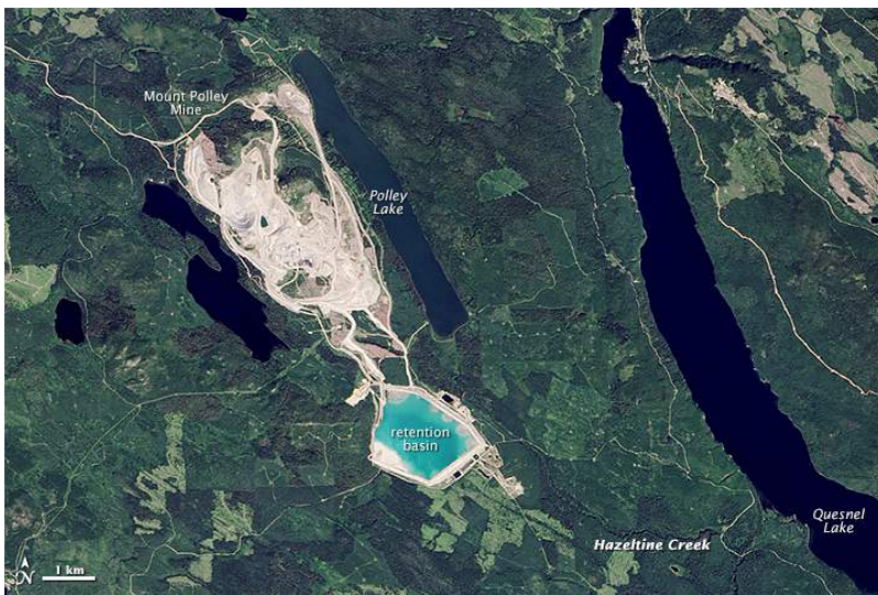
Figure 20.14a The Mt. Polley Mine area prior to the dam breach of August 2014. The tailings were stored in the area labelled “retention basin.” [ https://en.wikipedia.org/wiki/Mount_Polley_mine_disaster ]
