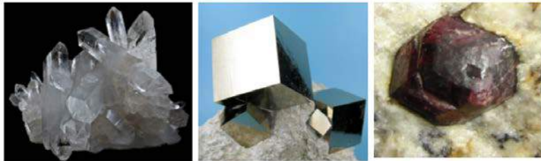
Figure 2.19 Hexagonal prisms of quartz (left), cubic crystals of pyrite (centre), and a dodecahedral crystal of garnet (right)
