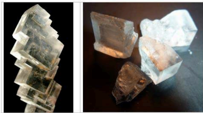
Figure 2.7 A depiction of the lattices of graphite and diamond. Figure 2.8 Cubic crystals (left) and right-angle cleavage planes (right) of the mineral halite. If you look closely at the cleavage fragment in the middle you can see where it would break again (cleave) along a plane parallel to the existing surface. Image on left: Halite by Rob Lavinsky, iRocks.com is under CC-BY-SA-3.0
