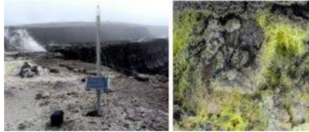
Figure 4.17 A gas-composition monitoring station (left) within the Kilauea caldera and at the edge of Halema'uma'u crater. The rising clouds are mostly composed of water vapour, but also include carbon dioxide and sulphur dioxide. Sulphur crystals (right) have formed around a gas vent in the caldera. [SE photos]
