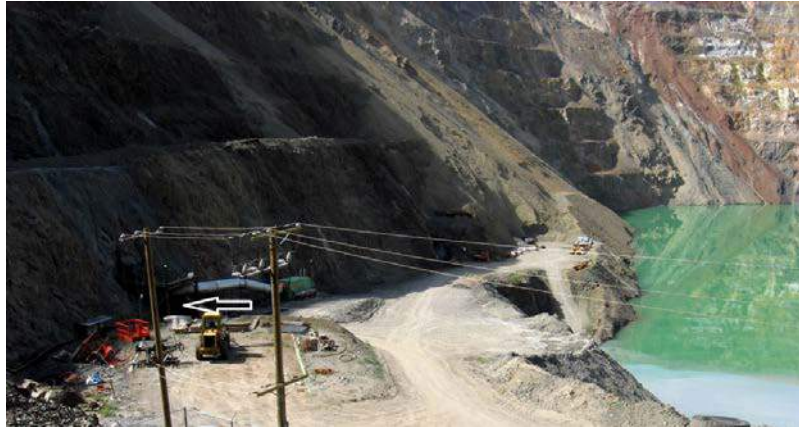
Figure 20.11 Entrance to an exploratory decline (white arrow) for the New Afton Mine situated in the side of the open pit of the old Afton Mine, near Kamloops, B.C. [SE]
