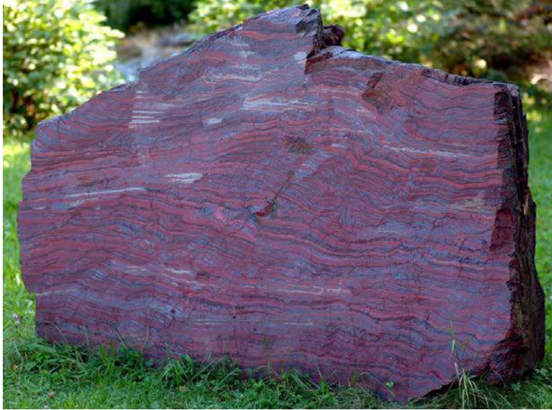
Figure 20.7 Banded iron formation from an unknown location in North America on display at a museum in Germany. The rock is about 2 m across. The dark grey layers are magnetite and the red layers are hematite. Chert is also present. [https://upload.wikimedia.org/wikipedia/commons/5/5f/Black-band_ironstone_%28aka%29.jpg]
