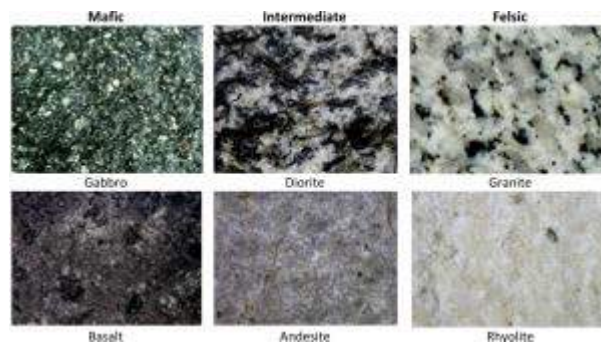
Figure 3.13 Examples of the igneous rocks that form from mafic, intermediate, and felsic magmas. [SE]
