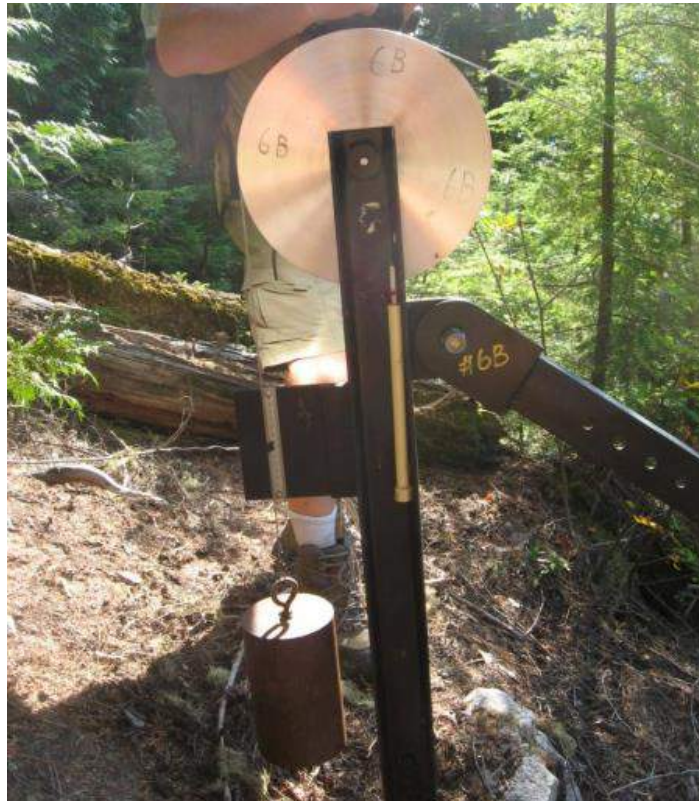
Figure 15.19 Part of a motion-monitoring device at the Checkerboard Slide near Revelstoke, B.C. The lower end of the cable is attached to a block of rock that is unstable. Any incremental motion of that block will move the cable, which will be detectable on this device. [SE]
