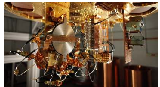
Figure 23.3: Superconducting quantum computer prototype at Google. Image credit: Google / MIT Technology Review.
