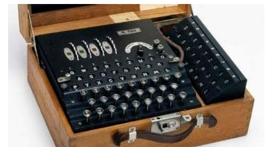
Figure 21.5: In the Enigma mechanical cipher the secret key would be the settings of the rotors and internal wires. As the operator types up their message, the encrypted version appeared in the display area above, and the internal state of the cipher was updated (and so typing the same letter twice would generally result in two different letters output). Decrypting follows the same process: if the sender and receiver are using the same key then typing the ciphertext would result in the plaintext appearing in the display.
