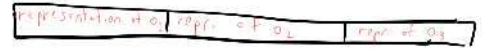
Figure 2.9: If we have a prefix-free representation of each object then we can concatenate the representations of k objects to obtain a representation for the tuple (o_0, \dots, o_{k-1}) .
