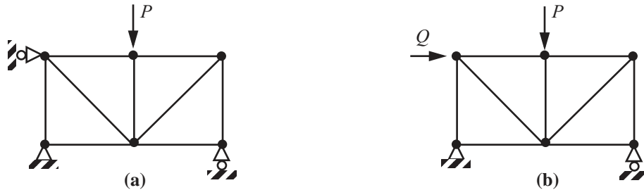
Fig. 6.17 A singly redundant truss (a), and its stable statically determinate base structure (b).
