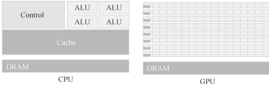
Fig. 1.6 CPU and GPU architecture
