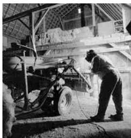
Front-end loader repair with Hobart 18AC stick electrode
