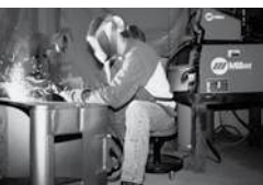
Welding fabrication using the Hobart Ironman 250 with Hobart HB-28 solid wire
