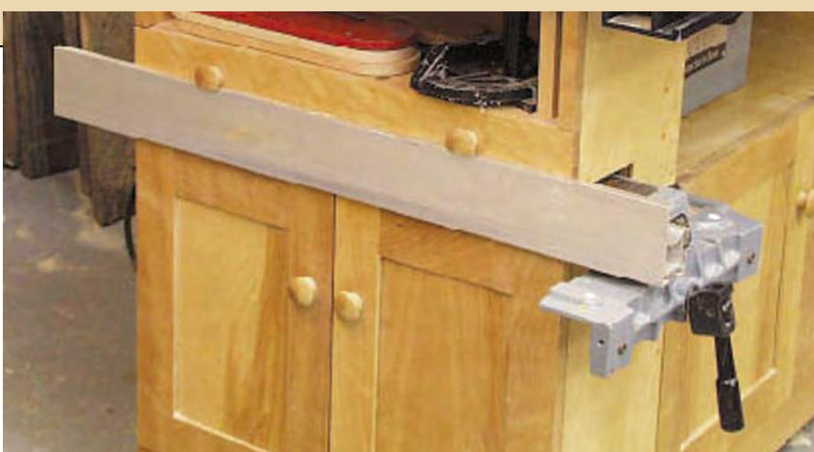
The saw cabinet offers plenty of storage, even a place to keep the fence when it's not in use.
