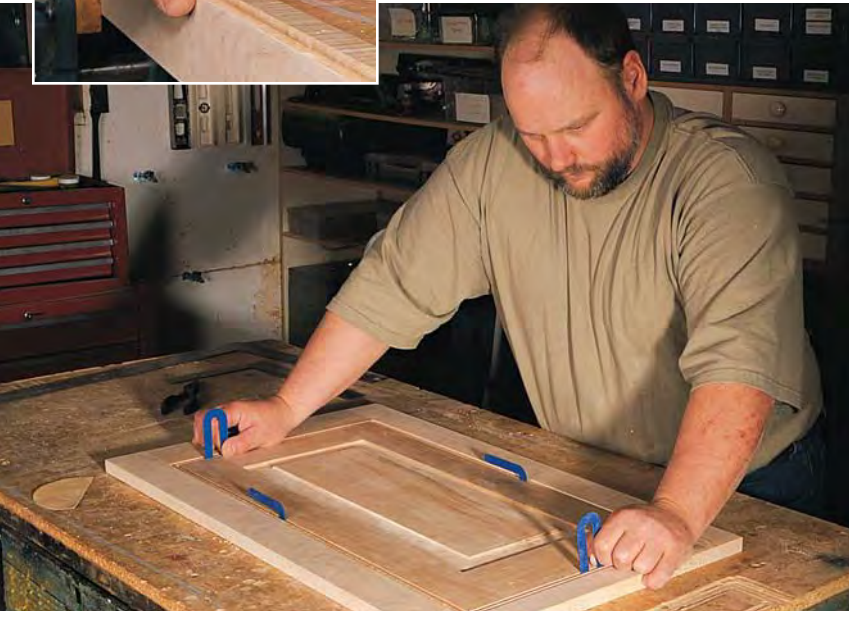
Fit your door in the face frame before you attach the face frame to the case. Everything lays flat on your bench as you work. You'll find this procedure is a faster and easier way to get perfect results.
