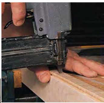
Adding this beaded moulding to the inside of the face frame creates a nice shadow line around the door. Miter, glue and nail it in place. Don't forget to putty your nail holes.
