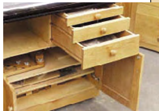
To make the odd-shaped cabinet, I attached three plywood boxes to each other. Each box has shelves and drawers for storage. The base box includes a dust collector.
