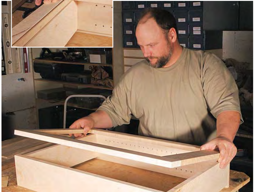
Fit the face frame on the case. The stiles should hang \frac{1}{16} " over the edge of the case so you can rout (or plane) them flush later.
