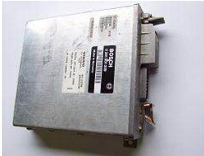
EDC control unit
