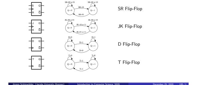
All flip-flops are edge triggered on the clock input C.
