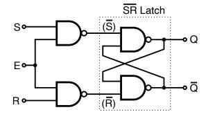
• The control input E enables the latch, the latch does not change while E is low.
