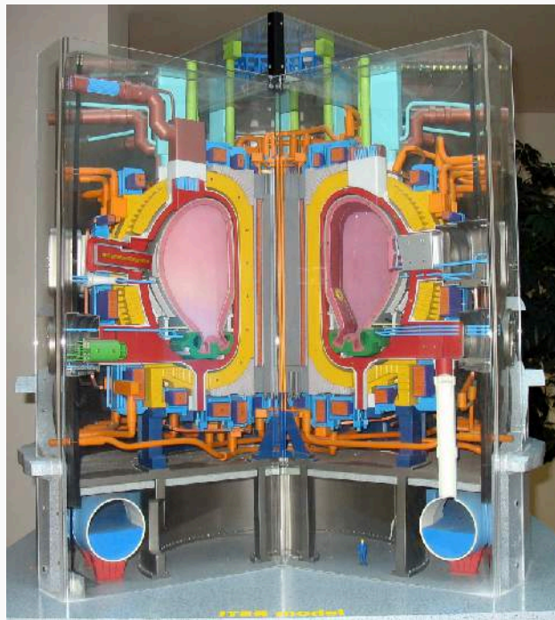
Figure 16.9 ITER Design. The bright yellow areas in this model show where the superconducting magnets will circle the chamber within which fusion will take place. A huge magnet will keep the charged nuclei of heavy hydrogen confined. The goal is to produce 500 megawatts of energy. (credit: modification of work by Stephan Mosel)
