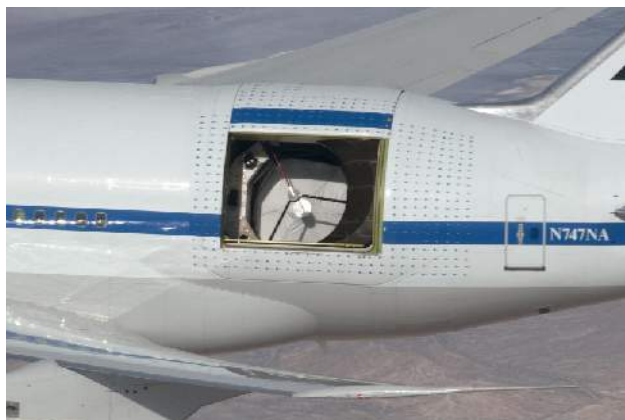
Figure 6.23 Stratospheric Observatory for Infrared Astronomy (SOFIA). SOFIA allows observations to be made above most of Earth's atmospheric water vapor. (credit: NASA)
