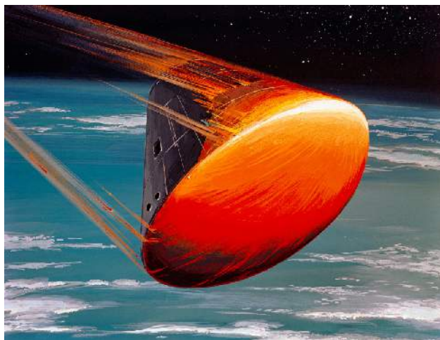
Figure 27.10 Friction in Earth’s Atmosphere. In this artist’s impression, the rapid motion of a spacecraft (the Apollo mission reentry capsule) through the atmosphere compresses and heats the air ahead of it, which heats the spacecraft in turn until it glows red hot. Pushing on the air slows down the spacecraft, turning the kinetic energy of the spacecraft into heat. Fast-moving gas falling into a quasar heats up in a similar way. (credit: modification of work by NASA)
