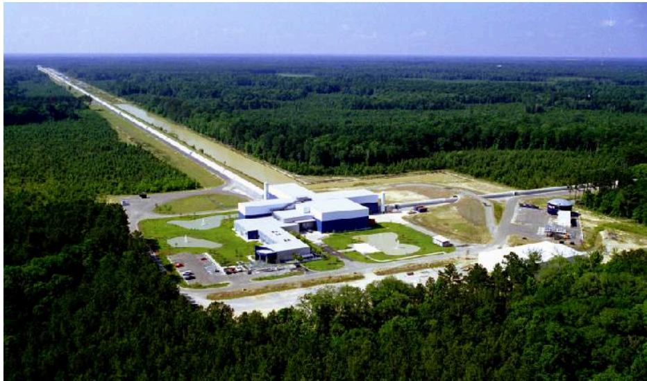
Figure 24.17 Gravitational Wave Telescope. An aerial view of the LIGO facility at Livingston, Louisiana. Extending to the upper left and far right of the image are the 4-kilometer-long detectors. (credit: modification of work by Caltech/MIT/LIGO Laboratory)
