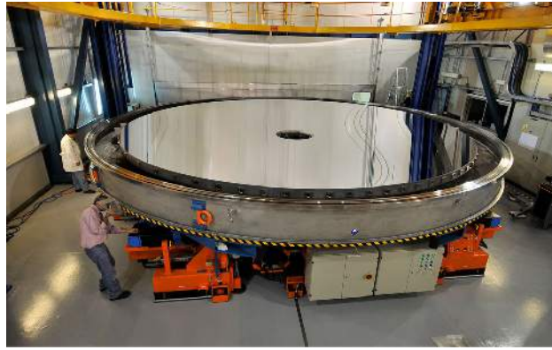
Figure 6.7 Large Telescope Mirror. This image shows one of the primary mirrors of the European Southern Observatory's Very Large Telescope, named Yepun, just after it was recoated with aluminum. The mirror is a little over 8 meters in diameter. (credit: ESO/G. Huedepohl)
