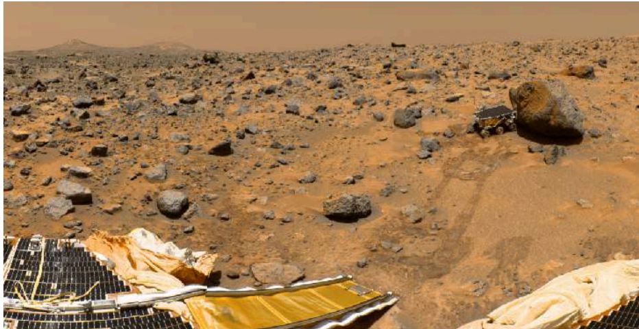
Figure 10.14 Surface View from Mars Pathfinder. The scene from the Pathfinder lander shows a windswept plain, sculpted long ago when water flowed out of the martian highlands and into the depression where the spacecraft landed. The Sojourner rover, the first wheeled vehicle on Mars, is about the size of a microwave oven. Its flat top contains solar cells that provided electricity to run the vehicle. You can see the ramp from the lander and the path the rover took to the larger rock that the mission team nicknamed “Yogi.” (credit: NASA/JPL)
