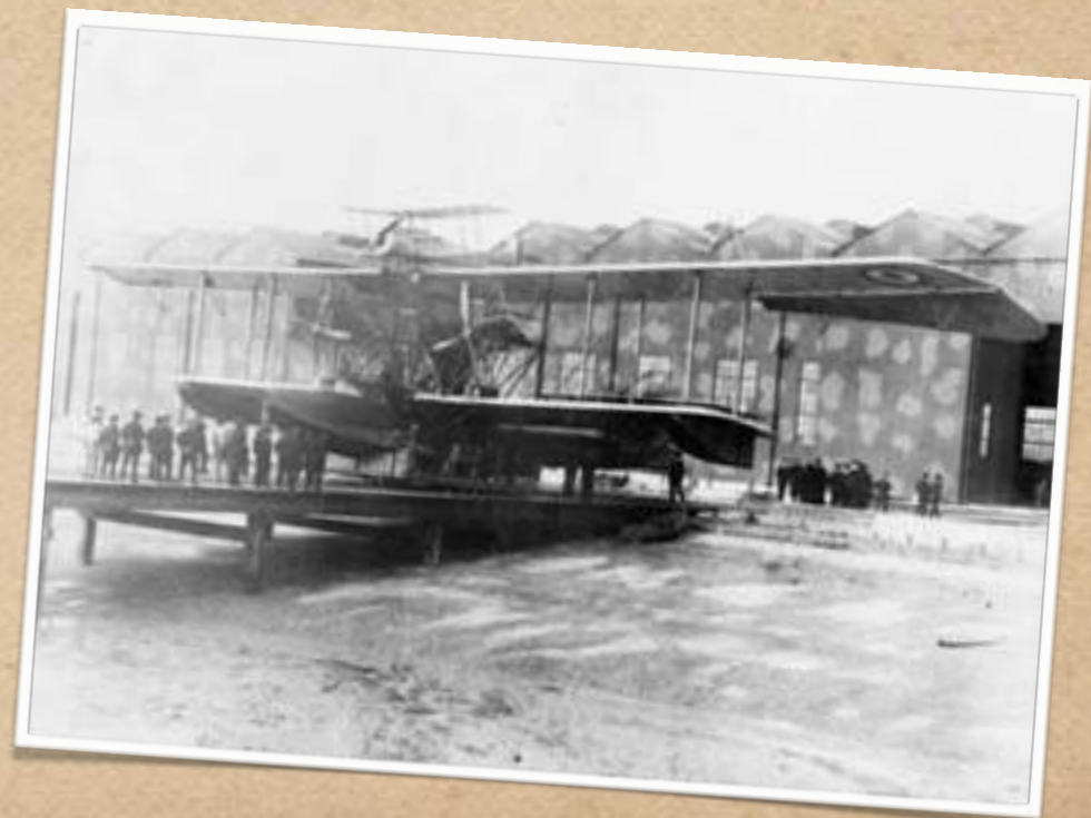
A Scout C on the upper wing of the Porte Baby flying boat at Felixstowe. IWM (Q 63768)
