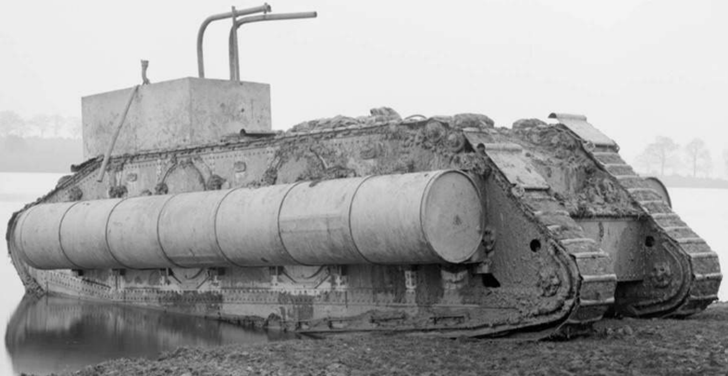
Flotation experiments with a Mark IX Tank at the Welsh Harp Reservoir, in Dollis Hill in London . IWM (Q 14625)
