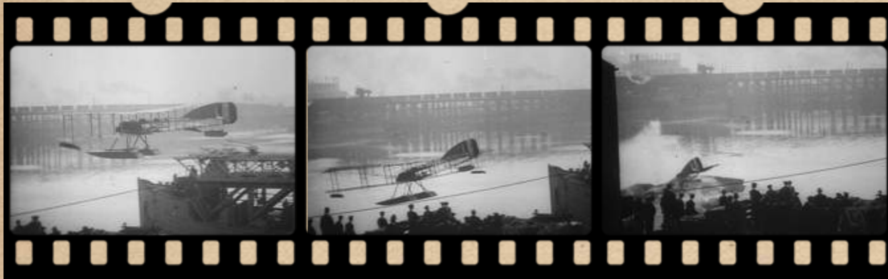
Launching seaplanes by catapult method from on board HMS Slinger in 1917. IWM (1166)
