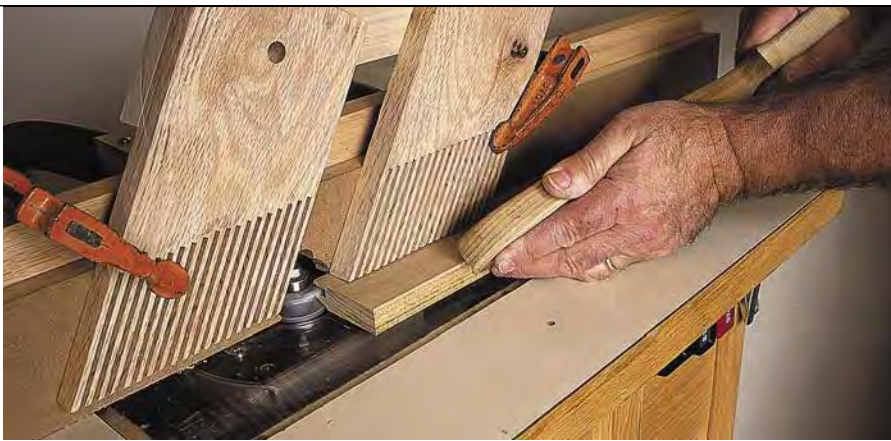
Make the sticking cuts by running the long edges along the fence. Featherboards will keep the stock flat on the surface of the router table.
