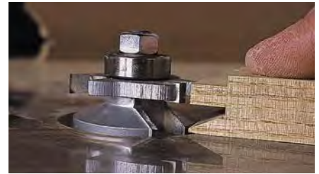
Use one of the coped pieces to set the height for the sticking cutter.
