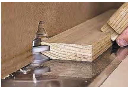
A zero clearance opening in the fence will help prevent chipping as the cuts are made.
