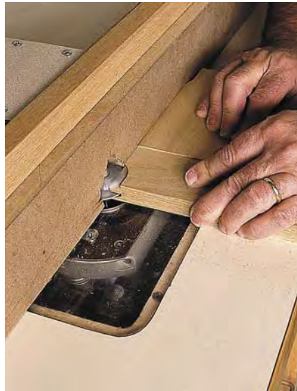
Use a block of scrap to push the end of the rail into the cutter for the cope. It will prevent tear-out and give you better control.
