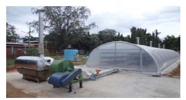
Renewable energy integrated drying system using solar thermal and biomass hot air with controlled environment can be used for continuous drying of agro-products.
