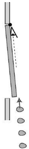
d / A putty blob thrown directly at the axis has no angular motion, and therefore no angular momentum. It will not cause the door to rotate.
