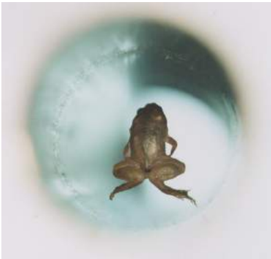
h / A frog is levitated diamagnetically by the nonuniform field inside a powerful magnet. Evidently frog has \mu < \mu_0 .
