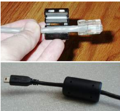
g / Example 25: ferrite beads. The top panel shows a clip-on type, while the bottom shows one built into a cable.
