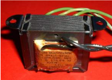
f / A transformer with a laminated iron core. The input and output coils are inside the paper wrapper. The iron core is the black part that passes through the coils at the center, and also wraps around them on the outside.
