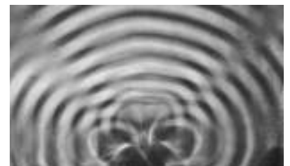
x / A pretty good simulation of the single-slit pattern of figure v, made by using three motors to produce overlapping ripples from three neighboring points in the water.
