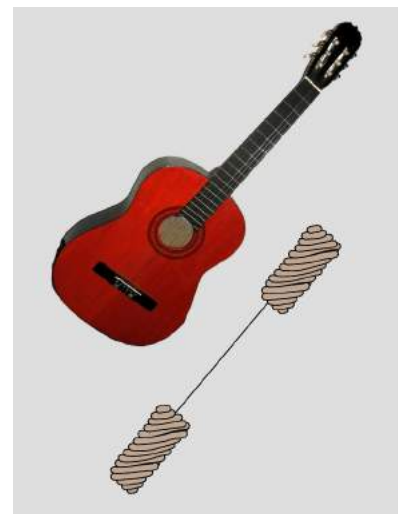
l / We model a guitar string attached to the guitar's body at both ends as a light-weight string attached to extremely heavy strings at its ends.
