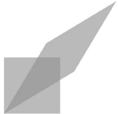
ai / A graphical representation of the Lorentz transformation for a velocity of (3/5)c . The long diagonal is stretched by a factor of two, the short one is half its former length, and the area is the same as before.
