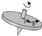
f / The position and momentum vectors of an atom in the spinning top.
