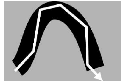
k / Total internal reflection in a fiber-optic cable.
