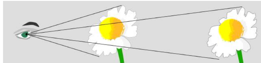
j / The angular size of the flower depends on its distance from the eye.
