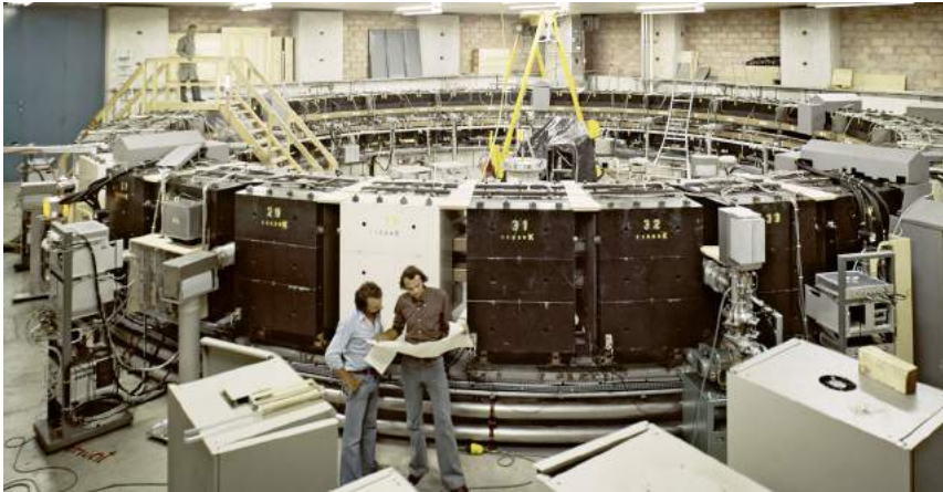
q / Apparatus used for the test of relativistic time dilation described in example 5. The prominent black and white blocks are large magnets surrounding a circular pipe with a vacuum inside. (c) 1974 by CERN.
