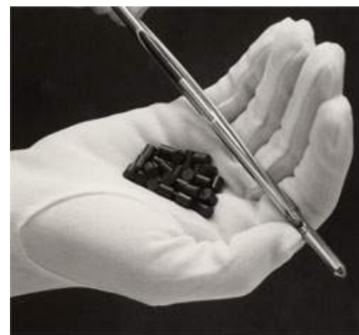
d / These pellets of uranium fuel will be inserted into the metal fuel rod and used in a nuclear reactor. The pellets emit alpha and beta radiation, which the gloves are thick enough to stop.
