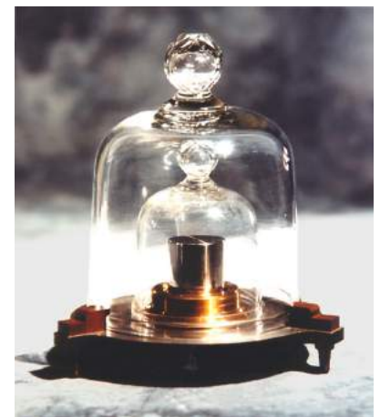
f / A duplicate of the Paris kilogram, maintained at the Danish National Metrology Institute. As of 2019, the kilogram is no longer defined in terms of a physical standard.
