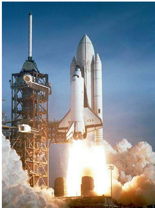
Figure 8.14 The space shuttle had a number of reusable parts. Solid fuel boosters on either side were recovered and refueled after each flight, and the entire orbiter returned to Earth for use in subsequent flights. The large liquid fuel tank was expended. The space shuttle was a complex assemblage of technologies, employing both solid and liquid fuel and pioneering ceramic tiles as reentry heat shields. As a result, it permitted multiple launches as opposed to single-use rockets. (credit: NASA)
