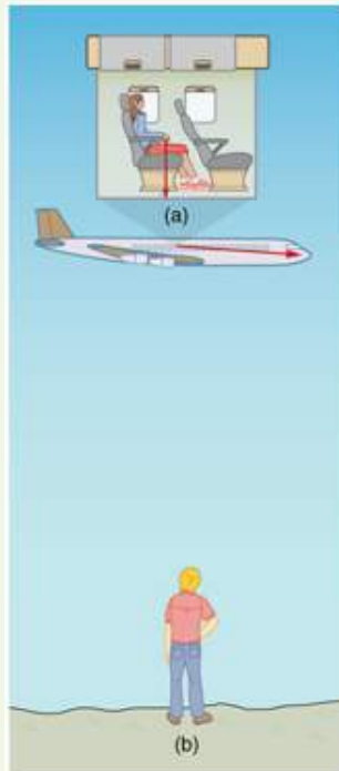
Figure 3.50 The motion of a coin dropped inside an airplane as viewed by two different observers. (a) An observer in the plane sees the coin fall straight down. (b) An observer on the ground sees the coin move almost horizontally.
