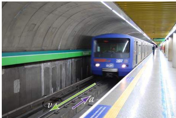
Figure 2.13 A subway train in Sao Paulo, Brazil, decelerates as it comes into a station. It is accelerating in a direction opposite to its direction of motion. (credit: Yusuke Kawasaki, Flickr)
