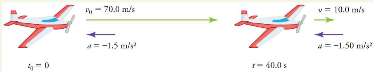
Figure 2.29 The airplane lands with an initial velocity of 70.0 m/s and slows to a final velocity of 10.0 m/s before heading for the terminal. Note that the acceleration is negative because its direction is opposite to its velocity, which is positive.
