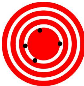
Figure 1.24 A GPS system attempts to locate a restaurant at the center of the bull's-eye. The black dots represent each attempt to pinpoint the location of the restaurant. The dots are spread out quite far apart from one another, indicating low precision, but they are each rather close to the actual location of the restaurant, indicating high accuracy. (credit: Dark Evil)
