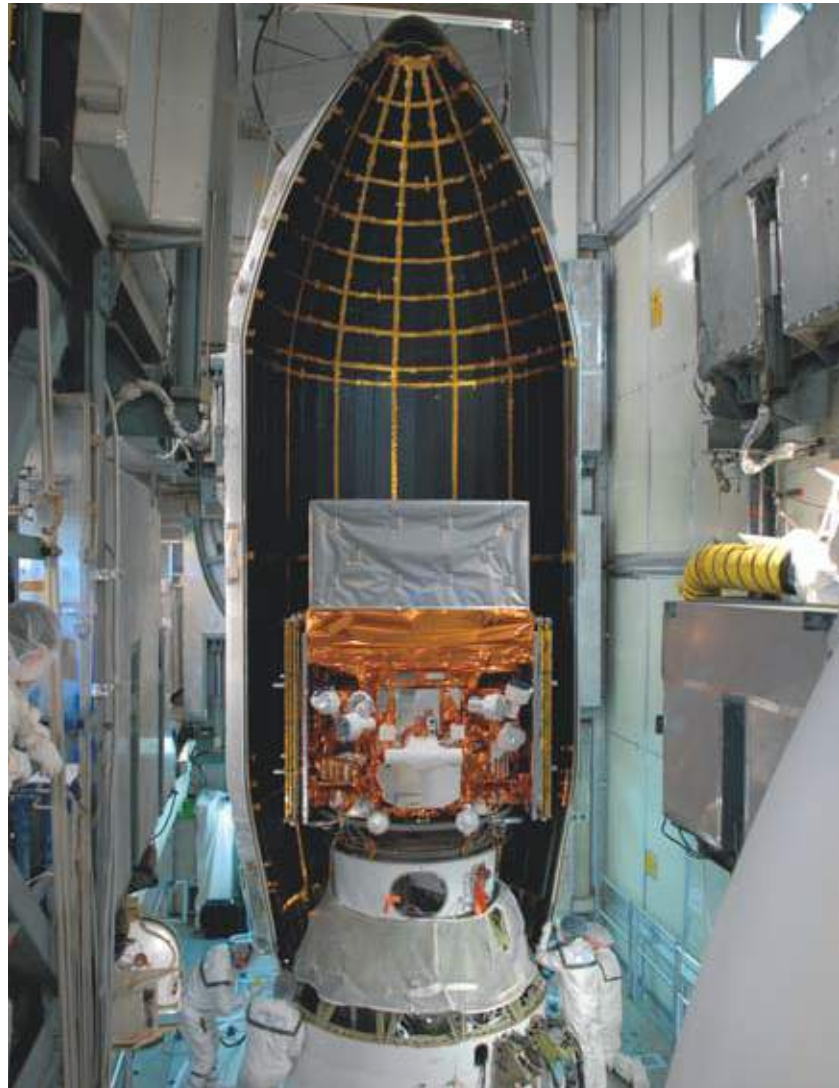
The Fermi observatory in its shroud, prior to being mounted on the launcher that placed it into orbit. NASA
