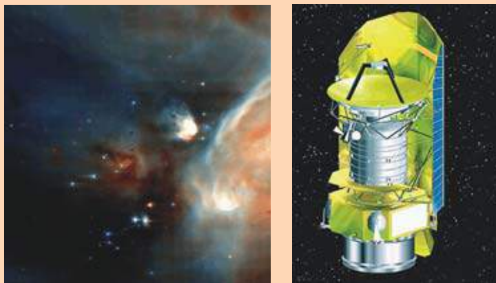
At right: artist's impression of the Herschel satellite, with the telescope and instrumentation positioned above a helium tank. Left: Herschel will be investigating star-forming regions in a hitherto unexplored energy range (image of Rho Ophiuchi, as viewed by the ISO satellite).
