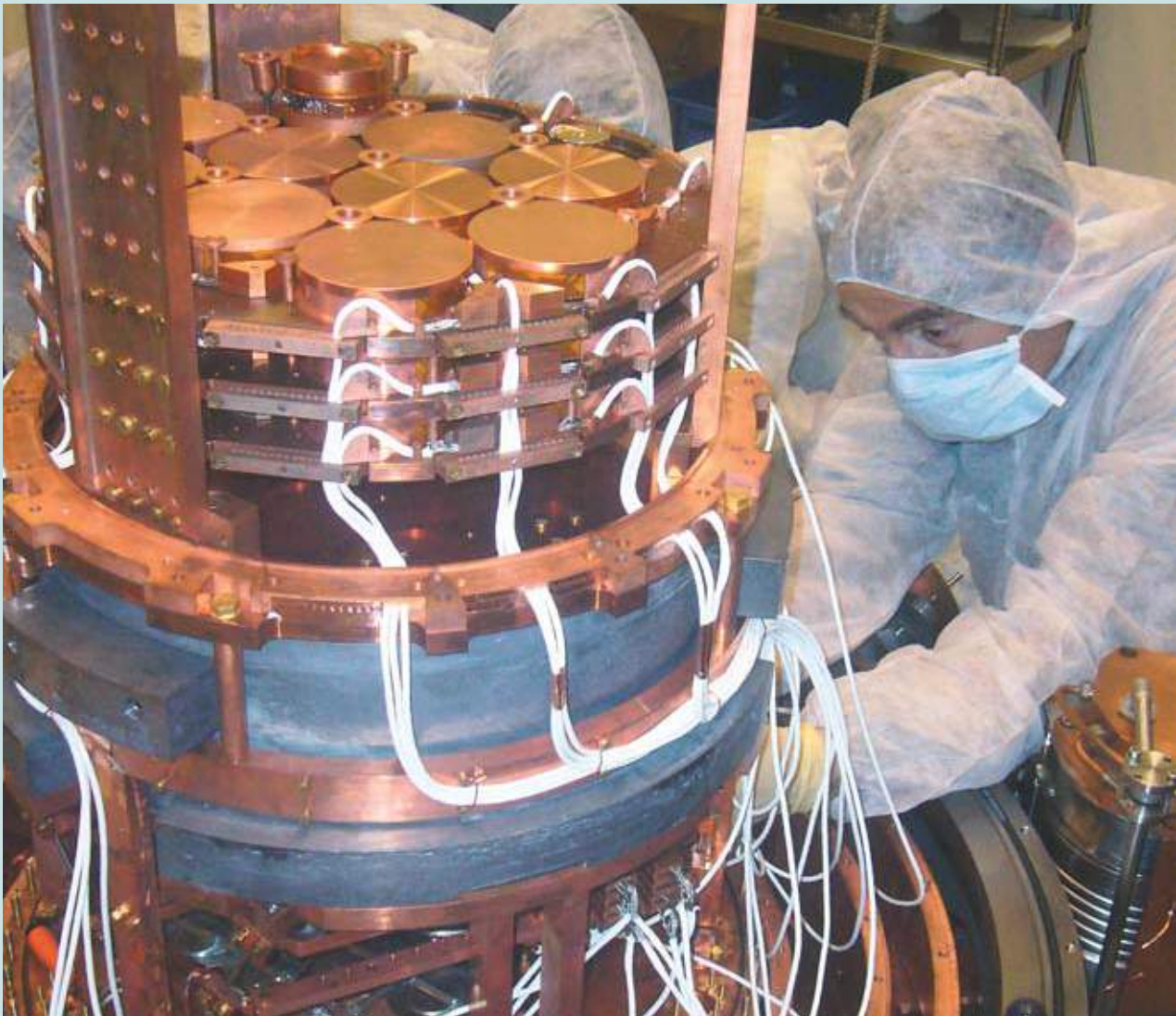
The EDELWEISS cryostat, standing open during detector mounting operations.
