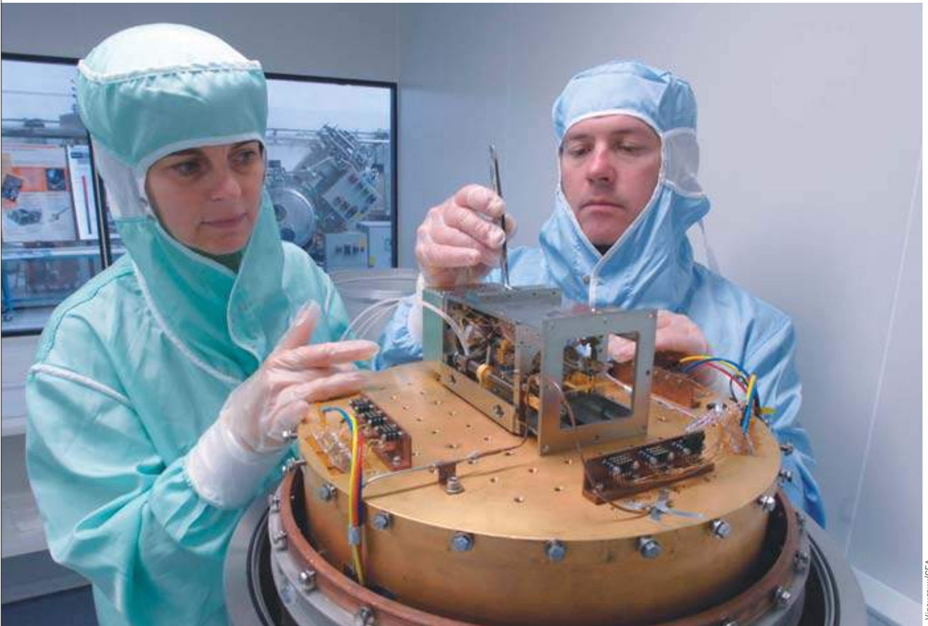
Setting up a flight cryocooler atop the test cryostat.
