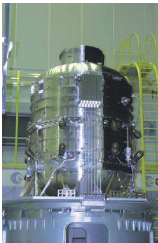
Herschel's cryostat holds 2,500 liters of helium, ensuring about 3 years' autonomy for the mission. This keeps the entire focal plane at a temperature of -271\text{ }^{\circ}\text{C} . As for the telescope, it is passively cooled to -200\text{ }^{\circ}\text{C} , by means of thermal shielding.
