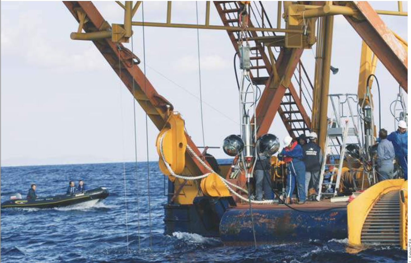
A storey, with its three “eyes,” being submerged during deployment of the first ANTARES line, 40 kilometers off La Seyne-sur-Mer, near Toulon (southern France).
