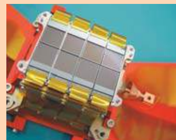
A bolometer is a kind of ultrasensitive thermometer, having the ability to detect minute variations in temperature (by a few millionths of a degree). Shown here, the bolometer-array (32 × 64-pixel) focal plane of the PACS instrument.
