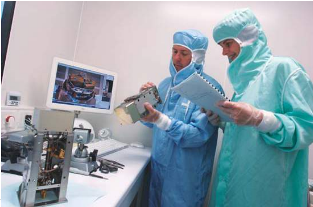
Work needs must be done on the issue of cooling the detectors carried on board satellites, so that they may operate correctly for ten years at least. Cryocoolers serve to cool detectors to a few hundred millikelvins. The picture shows thermal tests with the backup cryocooler for the Herschel satellite.
