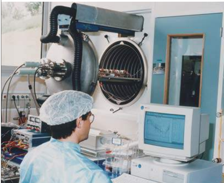
After takeoff, the satellite reaches the vacuum of outer space, exposed to heat from the Sun. Such conditions may be tested for, in a white room, on test models.
