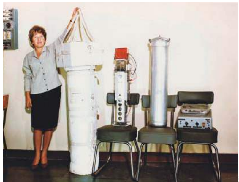
The payload carried by the balloon: detectors shielded from the vacuum in a leaktight pressure cooker, data being recorded on a tape recorder, recovered after the flight (May 1965).
