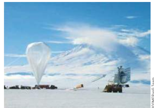
Figure 3. The launch, from an Antarctic base, of the BOOMERanG (Balloon Observations of Millimetric Extragalactic Radiation and Geophysics) stratospheric balloon, the forerunner to the OLIMPO experiment. Detection of the cosmic microwave background with OLIMPO will be carried out by means of four plane bolometer arrays, positioned at the focus of a 2.6-m diameter telescope.
