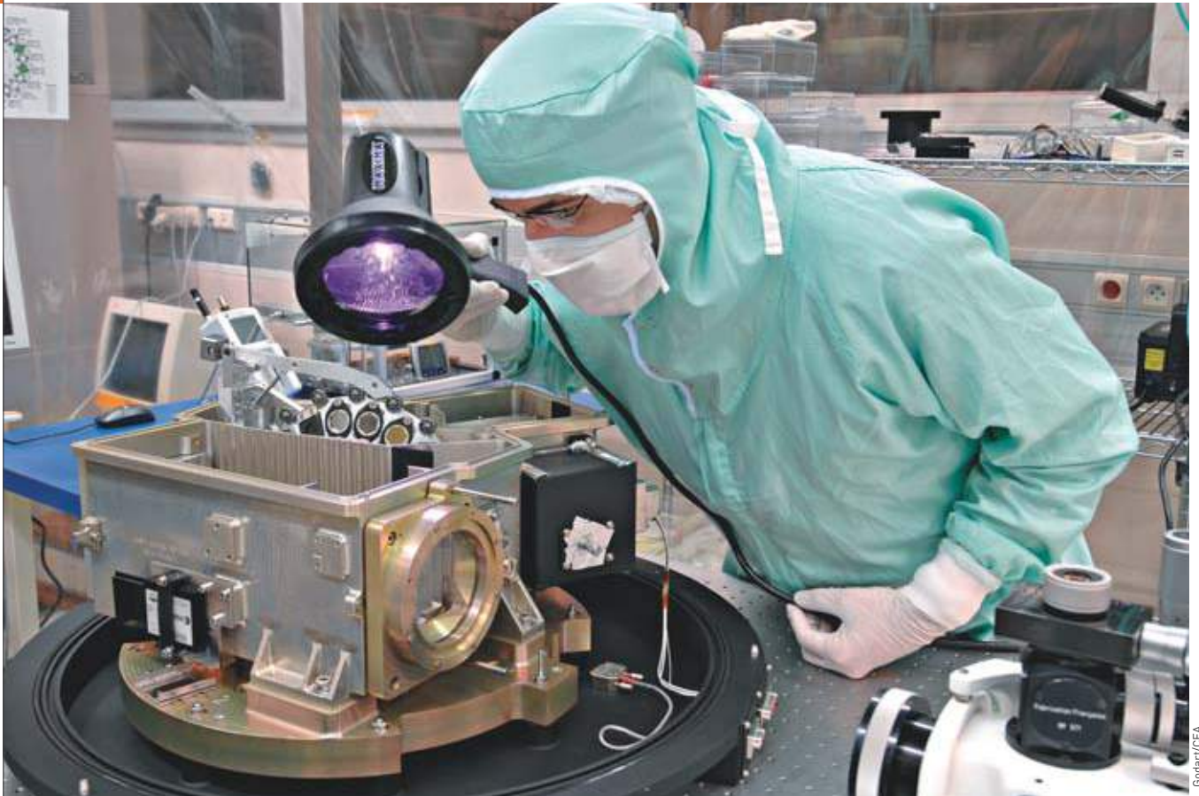
The Mid-Infrared Imager (MIRIM) camera, due to be mounted in JWST, being inspected, under ultraviolet light, to check no particulate contamination has occurred.
