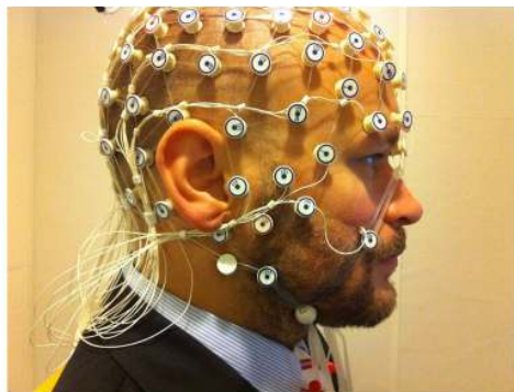
Figure 56.1. EEG recording setup. In an EEG, electrodes are placed on the head that can detect and record neuronal activity of the cortex.
