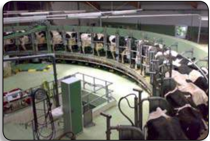
Dairy Cows being milked in a Rotary parlor
