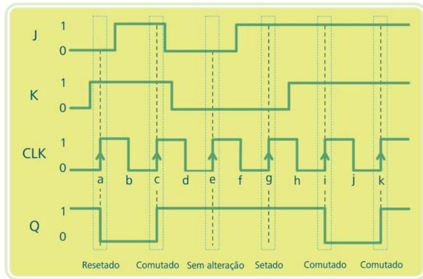
**Figura 4.21: Diagrama temporal do circuito sequencial**
