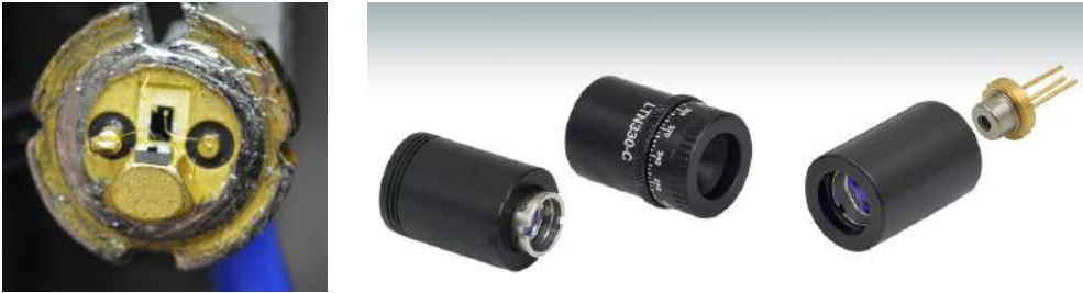
Figure 31.26: (Left) Laser diode with protective housing removed, e.g. using a can opener. (Right) Laser diode collimator.
