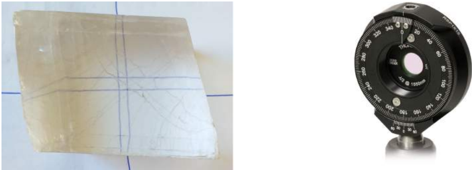
Figure 29.7: (Left) Transmission through a birefringent crystal. (Right) \lambda/2 -waveplate mounted in a rotation stage.
