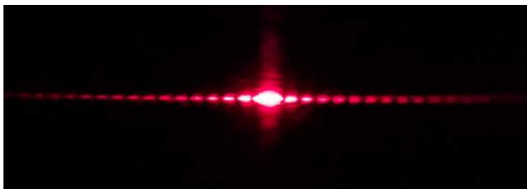
Figure 4. The interference of light waves through a double slit taken from this website .
