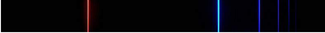
Figure 21. The Balmer m \rightarrow 2 series of the hydrogen spectrum, starting with the m = 3 line in red and then showing successive lines towards the ultra-violet.
