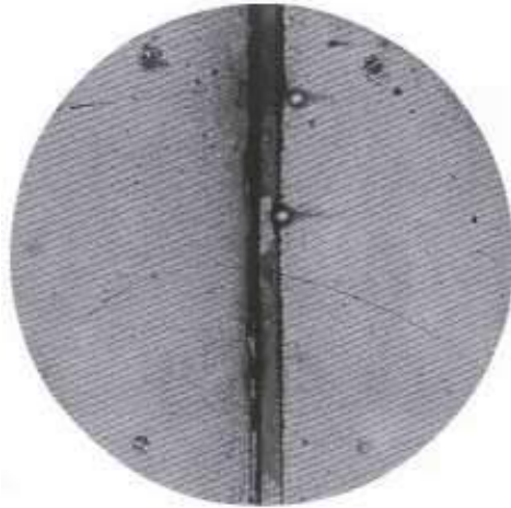
Figure 6.3: The first photograph of a positron ever taken in a cloud chamber. Note the curvature carefully. Which way is the particle travelling while slowing down? What direction does the magnetic field in the chamber point?
